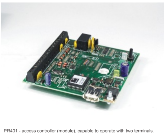
PR401 - access controller (module), capable to operate with two terminals.
